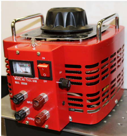
Figure 4.9: Power source for cartridge heater, VARIAC
